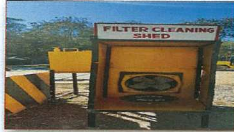
Filter Cleaning Shed: Filter cleaning shed is assembled departmentally in-house by the use of exhaust fan with assembly. The benefits are - • Reduction of dust emission during cleaning of used air filter of HEMM at garage premises.
