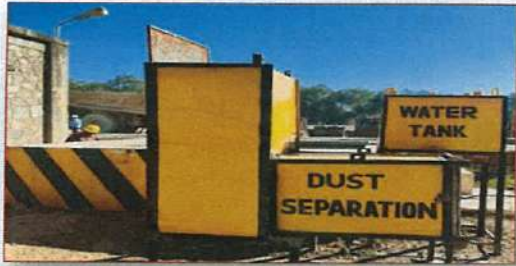
Filter Cleaning Shed: Filter cleaning shed is assembled departmentally in-house by the use of exhaust fan with assembly. The benefits are - • Reduction of dust emission during cleaning of used air filter of HEMM at garage premises.
