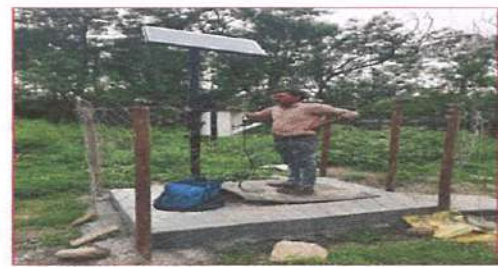
Ground water is being monitored for the wells around the lease area by establishing a network of four piezometer wells.
