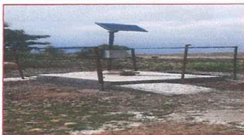
Ground water is being monitored for the wells around the lease area by establishing a network of four piezometer wells.
